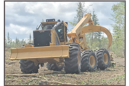
2019 TIGERCAT 625E 221 HP, 6WD. NEW Bogie Grapple Skidder. Excellent for soft terrain. . . . . CALL
